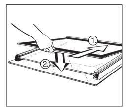
Insert the inner pane with the printed taxt facing downwards.
